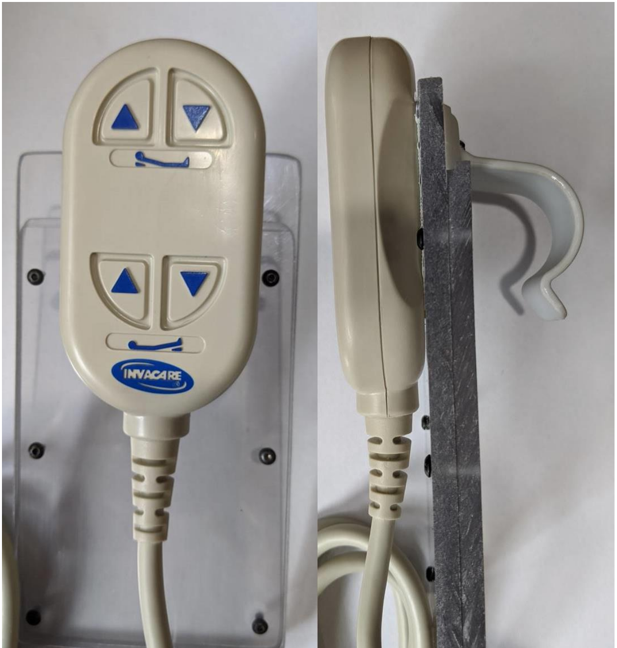
Figure 5 - Custom manual pendant using the Hill Rom hook to hang the assembly on the side rail.
