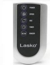
The Lasko fan remote sends an unknown format, so we captured the raw IR data and used that in a sketch that allows Kyle to control each feature by voice which then sends the raw IR data.
