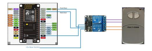
This is a two button Multi-Code remote that controls two different doors. GPIO 16 and GPIO 5 are used to energize the relays which then opens the appropriate door by closing the same contacts within the hand held remote as you would by depressing the button on the remote.
