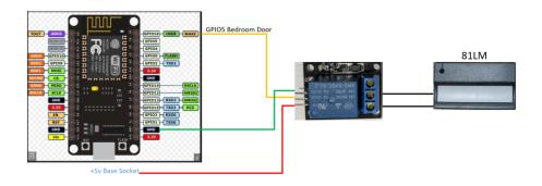
The Open Sesame door activation solution uses GPIO5 Pin D1 to energize the relay which then opens the Door by closing the same contacts within the hand held remote as you would by depressing the button on the remote. This single relay board requires a high trigger, so pinmode required in setup.
