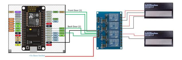
The Open Sesame door activation solution uses GPIO Pins 16 and 5 to open the Front Door, and GPIO pins 14 and 1 to open the Back Door. Inside each LiftMaster remote is a push button switch that is essentially double pole double throw. This required two GPIO and two corresponding relays for each door opener. The good news here is it offers redundancy since no single point of failure should result in unintended door opening.
