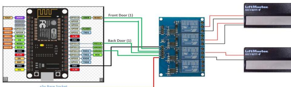
The Open Sesame door activation solution uses GPIO Pins 16 and 5 to open the Front Door, and GPIO pins 14 and 1 to open the Back Door. Inside each LiftMaster remote is a push button switch that is essentially double pole double throw. This required two GPIO and two corresponding relays for each door opener. The good news here is it offers redundancy since no single point of failure should result in unintended door opening.
