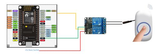
www.AdaptiveTechSolutions.com – Wireless Attendant Call Button part WDBA-FX-M-PLUG. (Remove Switch Adaptation = No You want the external 1/8" plug wired connection to connect to the relay. This solution could have also been done using a Smart Plug and a small relay box where the relay was configured to close n/o contacts on power up.
