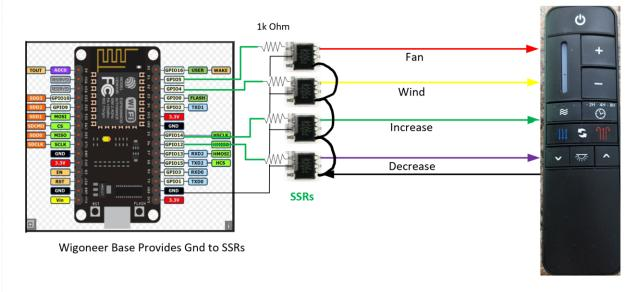
Remote – Soldered Connections to SSRs
