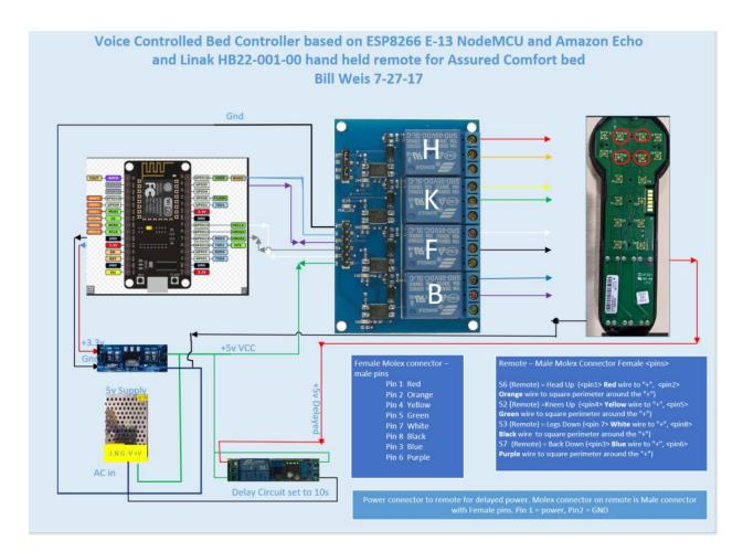
In the picture you can see the 4 relays labeled H, K, F, B (Head, Knees, Feet, Back). You can also see that I am providing power to the remote which normally has (3) AAA batteries. The object in the upper right is the remote with the plastic cover removed. The 4 red circles on the remote are where the relays are wired to. Silicone glue was applied to the board to provide strain relief for the newly soldered wires.
