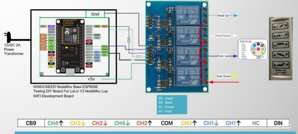
For safety reasons, lift/lower and Trend up/down are not controlled by voice, only head up/down and feet up/down are voice controlled. All functions are available using the standard pendant which is connected via a Y-cable so the voice controller and the hand held pendant can be connected at the same time.
